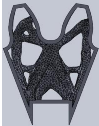
Figure. 6. The geometry of the gear's critical section in the ITOG model
