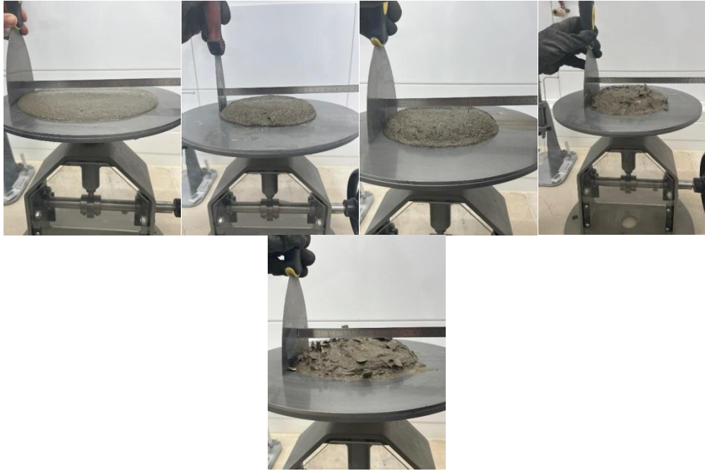
Fig. 3. Testing workability on specimens: RM, POW-1, POB-1, POW-2 and POW-3
